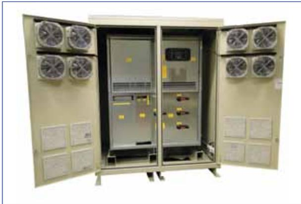
Harland Simon supplied their largest **Harland ProtectUPS® - Industrial** system to date incorporating a standard Riello 300kVA/60 minutes MHT AC UPS with fans and filters into an IP54 steel enclosure.
