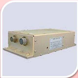
Harland Simon UPS designed a fully custom built military high specification DC power supply for an MOD ship radar.
