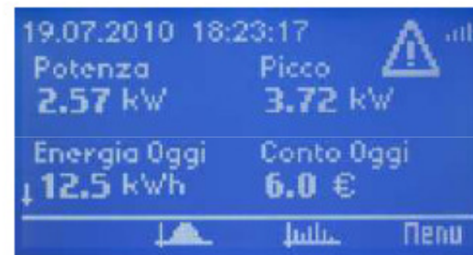
Alarm signal after audible warning alarm waiting for intervention
